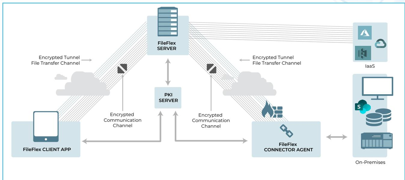
Diagram 1 - Zero Trust Architecture of FileFlex Enterprise
